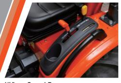
Hi/Low Speed Ranges The CX features a two range transmission (Hi/Low) to maximize performance and efficiency.
