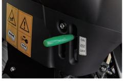
HST Linked Easy Speed When the HST linked pedal is engaged, the HST pedal and the engine rpm are synchronized. This reduces fuel consumption and simplifies tractor operation for a variety of utility and loader applications.
