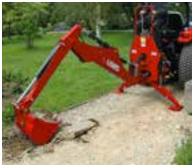
Boom and legs stabilise backhoe
