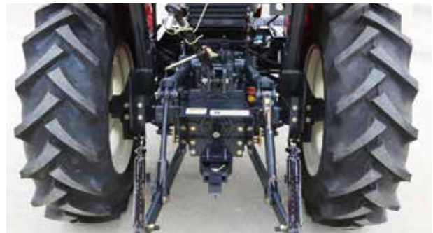
The Category I hitch has a lift capacity of 1,500kg at the ball end and 1,100kg measured 610mm behind the ball.
