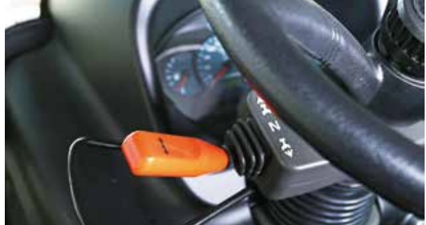
Power shuttle lever enables easy shifting between forward and reverse.
