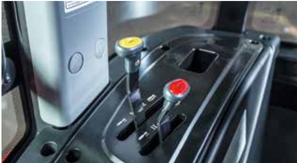
Conveniently located levers enable easy control of rear implements.
