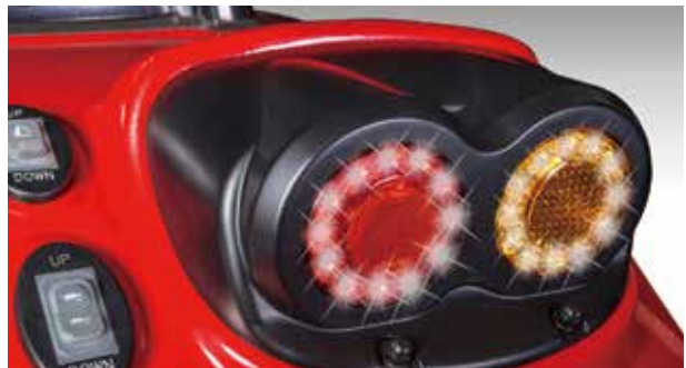
3PL lift arm control buttons are positioned on the rear fender and LED rear light is installed.
