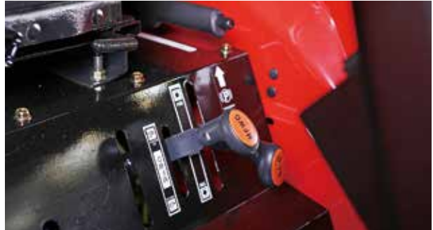
Differential lock system improves traction on slippery surfaces with easy accessible controls.
