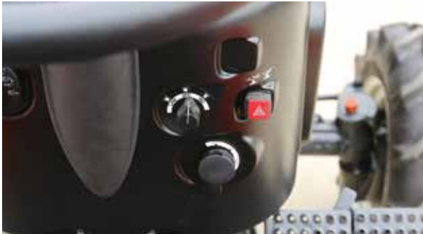
PTO operation : Electric Hydraulic Independent or Clutch linked.
