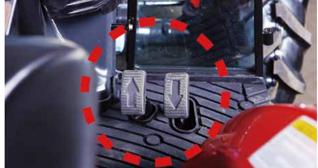
Hydrostatic control pedals for smooth hands free forward reverse motion HST models.
