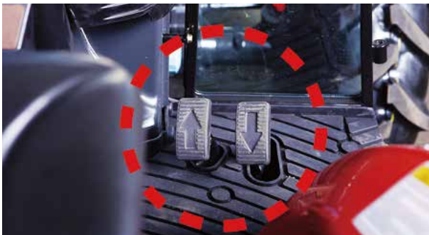
Hydrostatic control pedals for smooth hands free Forward reverse motion HST models.
