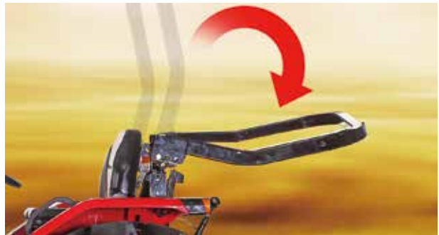
Foldable ROPS enables low clearance operation such as under trees.
