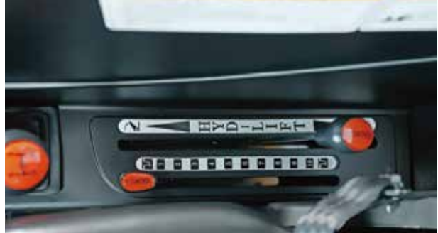
Three point linkage and draft controls for raising and lowering precision.
